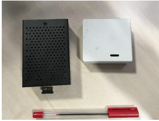
Figure 1: Sensor box (right) and gateway (left)
